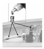
Unscrew the spring loaded valve and fill the boiler with the funnel approx. to the 3/4 (upper water gauge), if possible with warm water. The funnel should raise slightly so that the air can escape from the boiler. Use only deficient in lime water or, better, water without any lime e.g. distilled water.
